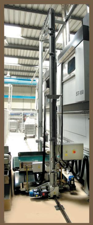
SHUTTLE LIFTING CONVEYOR WITH ONE OR TWO LOADING TABLES (CEDD or CEDS). APPROPRIATE FOR THE DISTRIBUTION OF LAUNDRY BATCHES FROM 1 TO 6 STATIONS.
