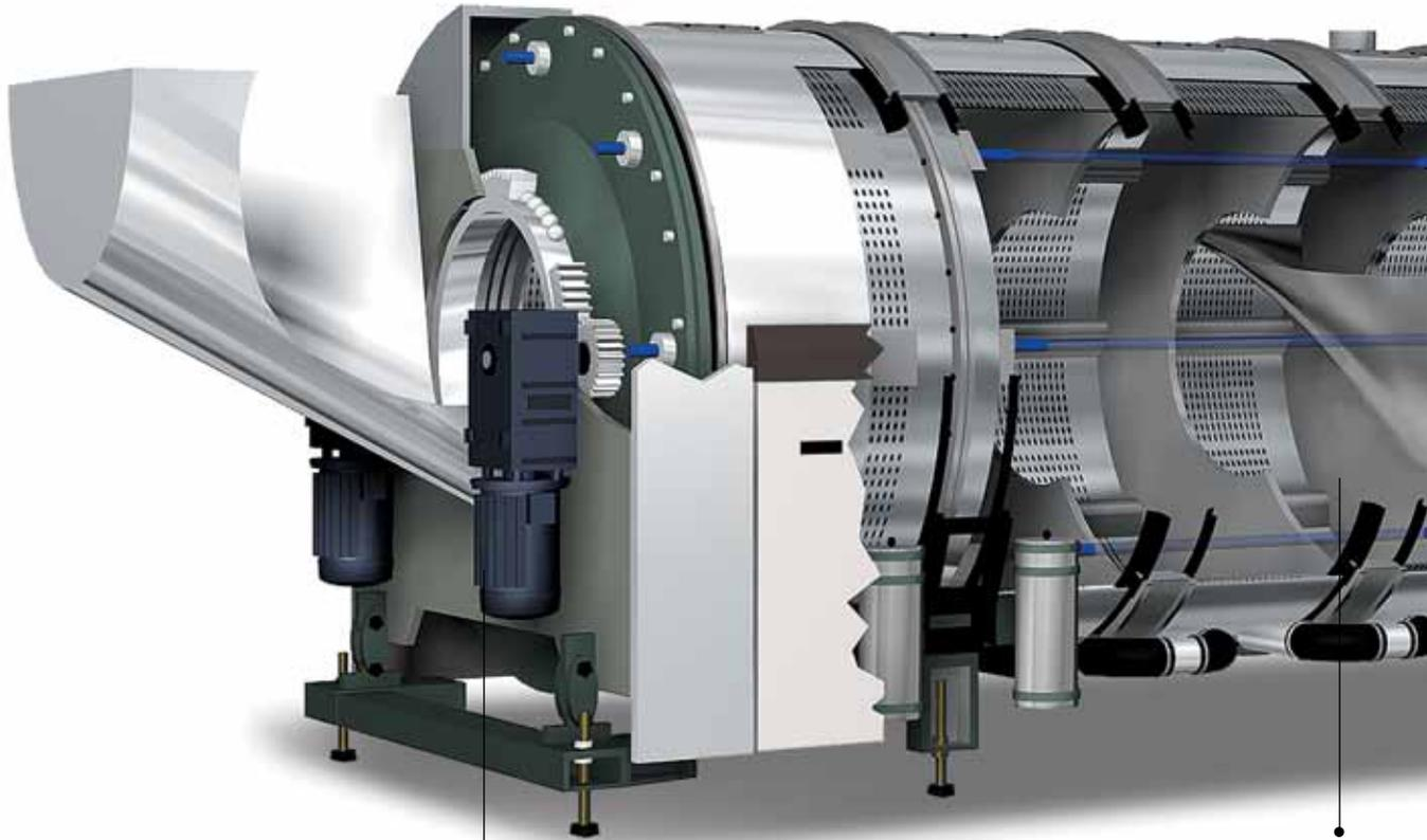
*The motor drive is located externally, away from moist areas to prevent damage. The transmission drive crown and sprocket are internally lubricated with no need for ongoing maintenance.*
